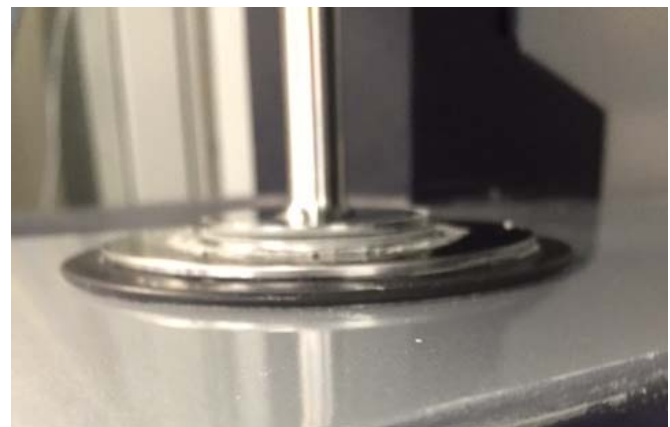
Figure 4: Close up of the Cone and Plate Mechanism
